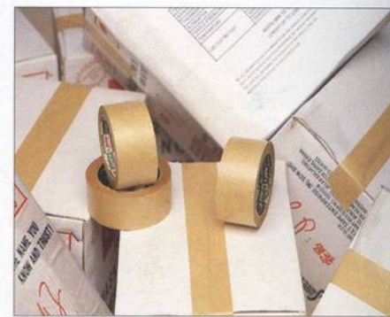
# R701/ # 701 S.K.P.T. Kraft Tape Main User: Sealing, Packing (Water Proof Tape) Standard Width: 12mm, 24mm, 36mm, 48mm, 96 mm Standard Length: 25m - 50m Thickness: ± 140mic Adhesive: Natural Rubber Latex (Emulsion)/ Acrylic Solvent
